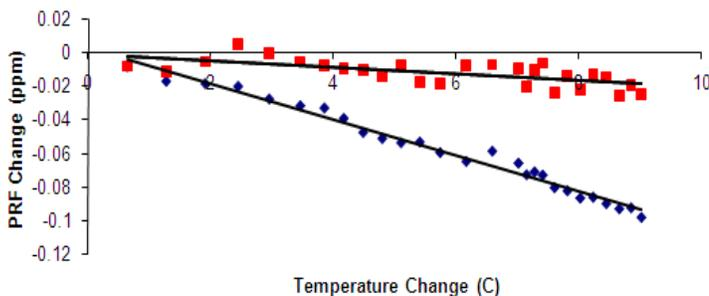
Figure 1: Temperature calibration performed via plotting the PRF of water (blue) and bulk methylene (red) versus measured temperature. The temperature sensitivity coefficient is the slope of the regression curve.
