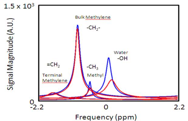
Figure 2: Measured spectra from one voxel in bone marrow at 17.2 °C (blue) and 34.8 °C (red) using the multi-gradient echo acquisition (ETL=16) at 3.0T with the SM algorithm (3). Terminal and bulk methylene, methyl, and water protons were detected and separated demonstrating multi-peak monitoring at high spatial and temporal resolutions ( $1.6 \times 1.6 \times 5.0$  mm<sup>3</sup>; 5 sec/image).
