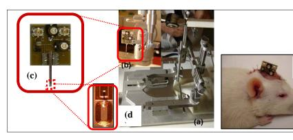
Figure 1. (a) Stereotaxy setup (David-Kopf), (b) Microcoil positioning, (c) Microantenna with tuning and matching circuit, (d) Needle-coil observed with scanning microscope (e) Rat equipped with microcoil.
