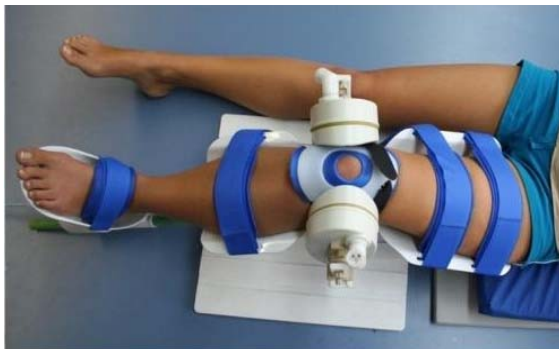
Fig. 1: Custom-made loading device with footplate for generation of compressive force on knee articular cartilage.
