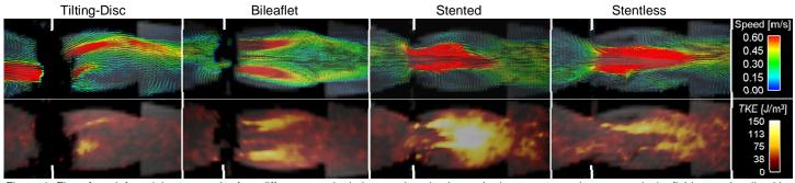
Figure 1. Flow, from left to right, across the four different prosthetic heart valves is shown. In the upper row, the mean velocity fields are visualized by streamlines, color-coded according to speed. In the lower row, turbulence maps color-coded according to turbulent kinetic energy (TKE) are shown. The white lines indicate the locations of the valves. Signal void caused by metal are seen the mechanical valves.
