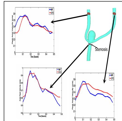
**Figure 1.** Comparison of maximum axial velocity between the CFD simulation and 4D MR flow imaging at three given cross-sections of a bifurcation aneurysm.
