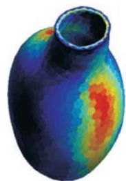
Figure 2 – Wall stress (red = high, blue = low)
