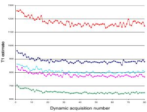
Figure 1. Short-term GRE signal drift for a selection of T1 samples. Each colour represents a different T1 sample (1210, 940, 786, 780, and 625 ms)
