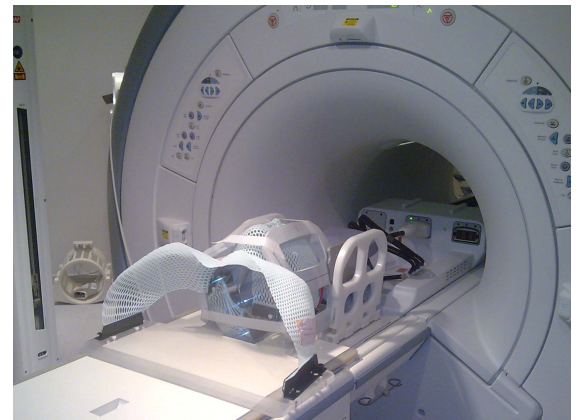
Figure 1. 4-channel cardiac coil wrapped around thermoplastic face mask containing test object.
