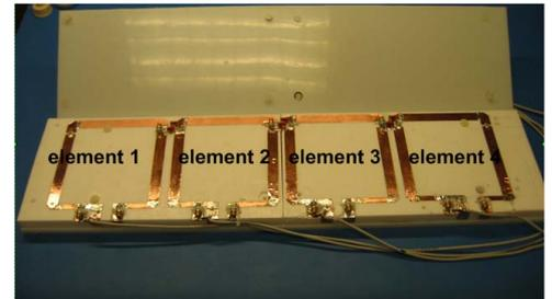
Fig.1 Photos of four-channel transceiver array at 7T.
