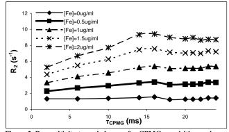
Figure 2.  $R_2$  sensitivity to varied  $\tau_{CPMG}$  for CPMG acquisitions using MPIO/gelatin samples with a range of iron concentrations. Diffusion sensitivity is consistent with Luz-Meiboom predictions.
