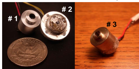
Figure 1. ICP devices. The casing material of device #1, #2, and #3 were stainless-steel, aluminum, and titanium, respectively.
