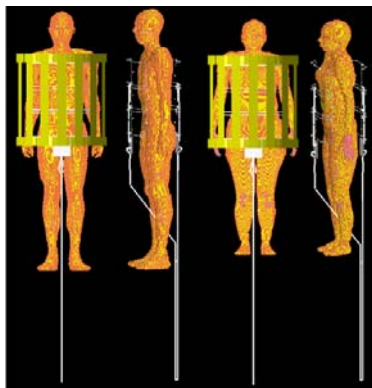
Fig. 1. The human body model and coil geometry (shield hidden). Left two are front and side (birdcage coil hidden) view of NORMAN. Right two are front and side view of NAOMI
