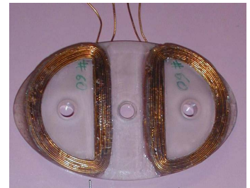
Fig. 3 Gradient coil: radius of the wrapping is 35 mm and the gap between them is 16 mm.
