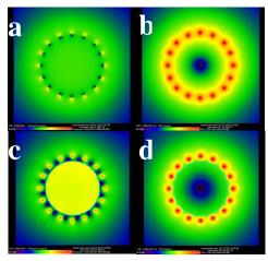
Fig 1.  $\mathbf{B_1}^*$  magnitude distribution without(a) and with(c) high dielectric insert.  $\mathbf{E}$  magnitude distribution without (b) and with(d) high dielectric insert
