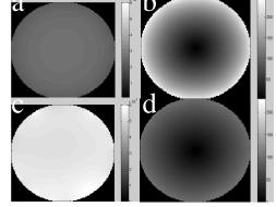
Fig 2.  ${\bf B_1}^*$  magnitude distribution within ROI without(a) and with(c) high dielectric insert.  ${\bf E}$  magnitude distribution within ROI without (b) and with(d) high dielectric insert
