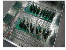
Figure 3. Amplifiers on motherboards inside a rack mountable enclosure.
