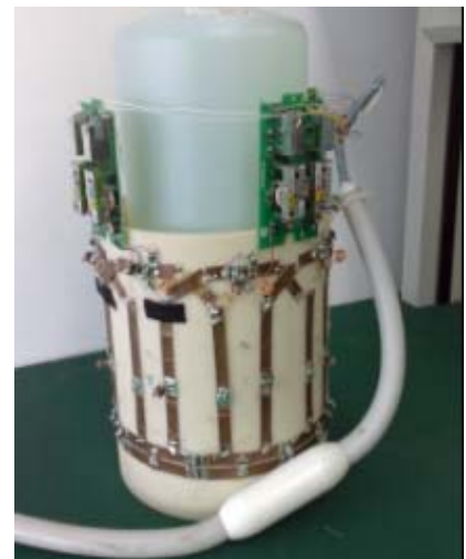
Fig.3 8-channel coil with a phantom
