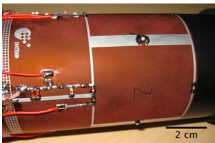
Fig 1. Four-channel receive coil array on flexible substrate, wrapped around a thin-walled PEEK cylinder.
