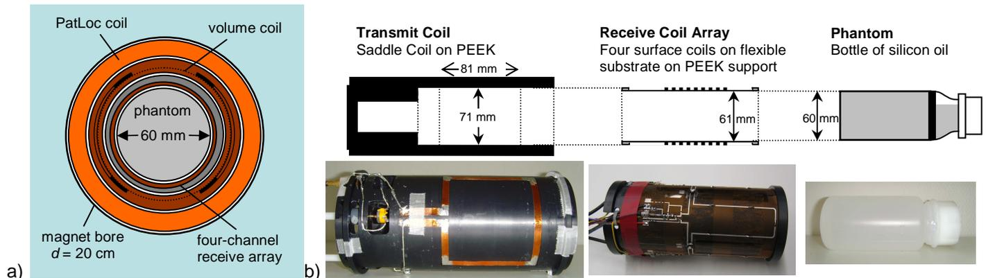
Figure 1: (a) Sketch of cross-section of arrangement of gradient coils, RF transmit and receive coils inside of a 9.4 T magnet with phantom of diameter  $d = 6$  cm; (b) Sketch and photos of side view of four-channel coil
