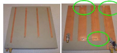
Fig. 2. Microstrip-coax design: Left - imaging side; Right - ground plane and coax sections (green circles).
