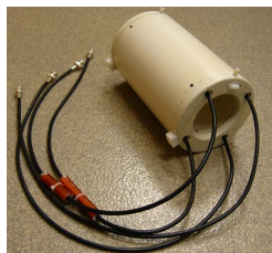
Fig.1 16-element double-tuned birdcage with Diameter=4" and Length=5"
