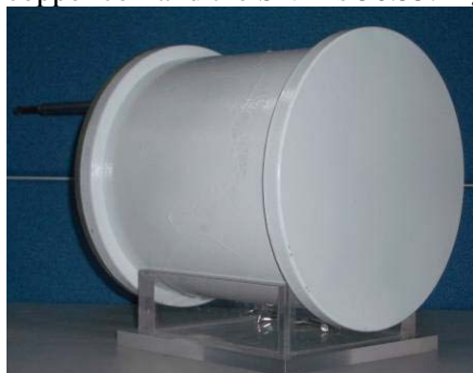
Fig.1. LN 2 based cryostat
