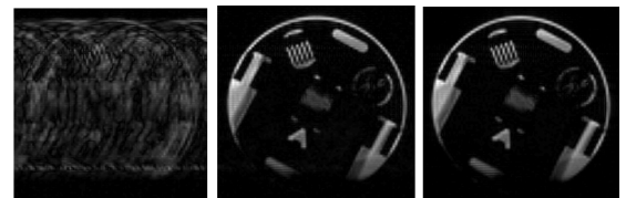
Fig.3 Gradient echo images (256x128) acquired with the self-made data acquisition system (leftmost) and GE Signa 12M4 receiver (rightmost). The phase in-coherency with the self-made receiver is compensated in the center image.
