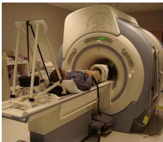
Fig.1 MRI-compatible load-bearing apparatus
