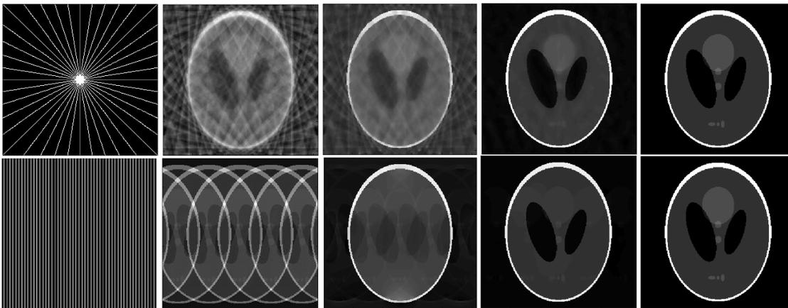
Fig. 2: Exact reconstruction of the Shepp-Logan phantom using samples in k-space given by the leftmost columns. Subsequent columns are progressive iterations of the algorithm which produce an exact reconstruction.
