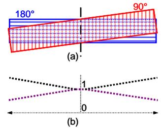
**Figure 1:** (a) Slice orientation during 90° and 180° RF pulses; (b) Theoretical profile of signal loss in the phase-encoding direction (in purple), and the kernel for intensity correction (in black).
