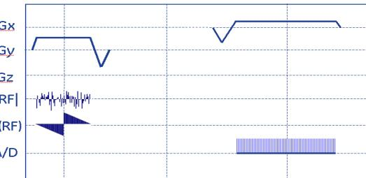
Figure 1. Timing diagram of the pulse sequence for Toeplitz random encoding.
