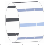
Fig. 1: Schematic drawing of the RF coil used in this study: The coil consist of 3 segments with 8 elements each.
