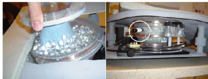
**Figure 1.** (left) Chicken breast within a surgical glove was placed within the coil and surrounded by small beads to provide uniform pressure around the entire surface area of the breast. (right) Lateral view of a biopsy needle insertion through the beads into the tissue (white circle). The three conductor turns of the solenoid coil are also visible.
