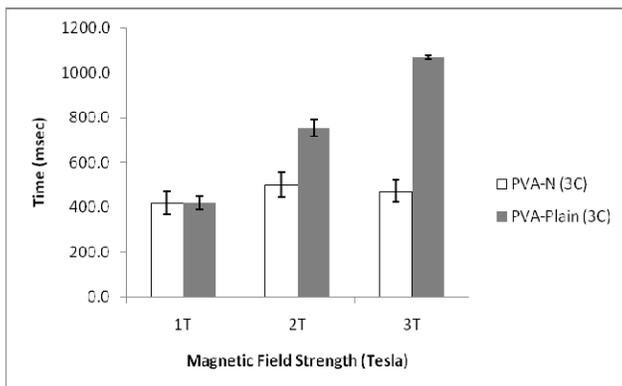
Figure 1 –  $T_1$  Relaxation Times for PVA at 1, 2 & 3T
