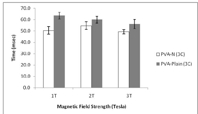
Figure 2 –  $T_2$  Relaxation Times for PVA at 1, 2 & 3T
