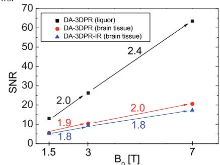
Fig. 4. SNR values of the DA-3DPR images shown in Fig. 3 and of the DA-3DPR-IR images. The numbers on the arrows indicate SNR increase from 1.5 T to 3 T and from 3 T to 7 T.
