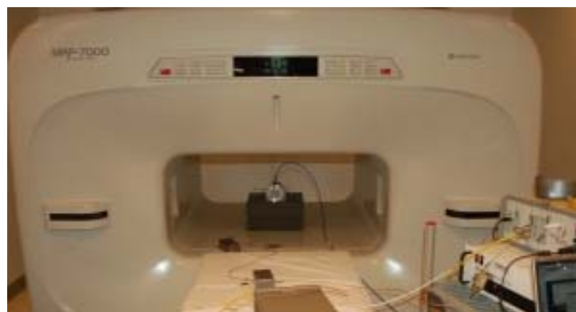
Figure 2: A DNP experiment using a clinical 0.3T MRI magnet, using portable NMR and DNP equipment.
