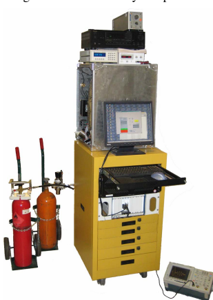
Figure 1: The PASADENA polarizer, with reaction chamber in silver case, electronics in yellow case, and attendant parahydrogen and nitrogen gas cylinders.
