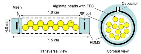
**Figure 1:** Coil-construct assembly schema. The macroconstruct consists of a coil surrounded by PDMS and containing alginate beads with perfluorocarbonate (PFC).
