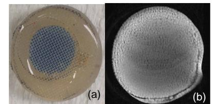
**Figure 2:** (a) coil-construct assembly with blue-colored beads within the cavity; (b) NMR image of the cavity containing cell-free BaA beads *in vivo* with an in-plane resolution of 78  $\mu$ m.
