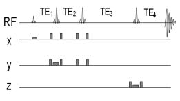
Fig. 1 Pulse sequence of modified PRESS using four RF pulses for glutamate editing pulses.
