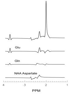
Fig.2. Simulated four-pulse PRESS spectra of NAA, glutamate and glutamine. TE = 94 ms, TE<sub>1</sub> = 14 ms, TE<sub>2</sub> = 15 ms, TE<sub>3</sub> = 33 ms, TE<sub>4</sub> = 32ms. 1st trace: summed spectrum; 2nd trace: glutamate; 3rd spectrum: glutamine; 4th spectrum: aspartate moiety of NAA.
