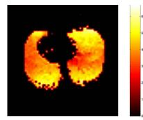
Fig. 3.  $B_1 \alpha^{\circ}$  map from a 2 cm axial slice, the coil transmit inhomogeneity is evident.
