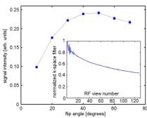
Fig. 4. SNR of SSFP as a function of flip angle in the phantom experiments. The optimum SNR occurs for  $\alpha = 50^{\circ}$  which is larger than was optimised for a longer TE (5 ms) symmetric echo SSFP sequence at 1.5T [1]. The shorter TE used here limits diffusion attenuation of the transverse magnetisation and thus permits a higher flip angle. Inset is the typical k-space filter as a function of
