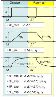
**Fig. 1:** Six different model functions with 2 to 5 free parameters (rel. enhancement c; time delays  $\Delta t$ ,  $\Delta t$ '; wash-in and wash-out times  $\tau_1$ ,  $\tau_2$ ) were compared for pixelwise fitting of  $O_2$ -MRI data.
