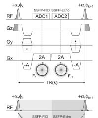
Fig. 1 (top): Partially spoiled dual echo steady state (pDESS) sequence scheme. The difference between consecutive RF phases is linearly incremented. (bottom): The ADC for the two echoes must be gauged to the phase of the corresponding RF pulse.
