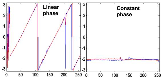
Fig 1. Linear (left) and constant (right) phase correction parameters obtained in a phantom from the dual reference scans for imaging frequency set to the water (blue) and fat (red) resonances.
