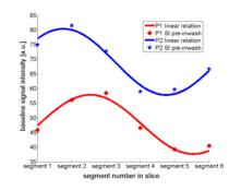
Figure 2: The linear relation before inwash of contrast agent is shown for two patients at rest. Spatial linearity in signal intensity across segments in a circle results in a sinusoid. The dots are the actual pre-inwash signal intensities of the baseline signals per segment.
