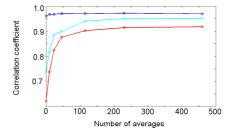
Figure 3: Correlation coefficient comparing median nerve response signal with EEG signal from Pz as a function of number of averages without gradients and pulses (blue); for uncorrected data recorded with R-peak timed pulses (red); and for pulse artefact and baseline corrected data (cyan).
