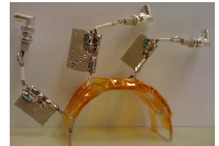
Fig. 1: Dedicated 3-element array (before packaging).
