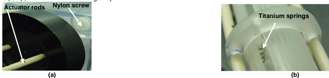
Figure 2: (a) MR compatible plastic equivalents in bioreactor design and b) MR compatible Titanium springs for sample attachment
