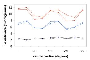
Fig 2 Iron estimate based on black volume on TE=25ms image (top), 10 ms (middle) and phase difference (bottom). Solid and hollow symbols have read and phase axes interchanged.
