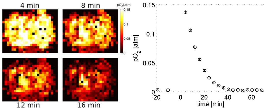
**Figure 2:**  $p\text{O}_2$ -images of a cross-section of a hemodialysis filter at four subsequent times post  $\text{O}_2$ -injection.  $^{19}\text{F}$   $T_1$ -images, recorded with a fast  $T_1$  sequence on a 3T scanner, were used to calculate the  $p\text{O}_2$ -images.
