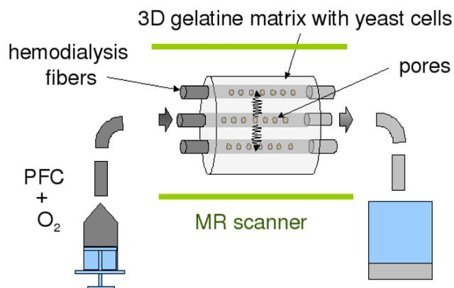
**Figure 1:** The dialysate compartment of a hemodialysis filter was filled with a gelatine matrix containing viable yeast cells. An oxygen rich perfluorocarbon (PFC) was pumped through the fibers of the blood compartment of the hemodialysis filter, using a syringe. The entire setup was positioned in a Siemens Trio 3T scanner.
