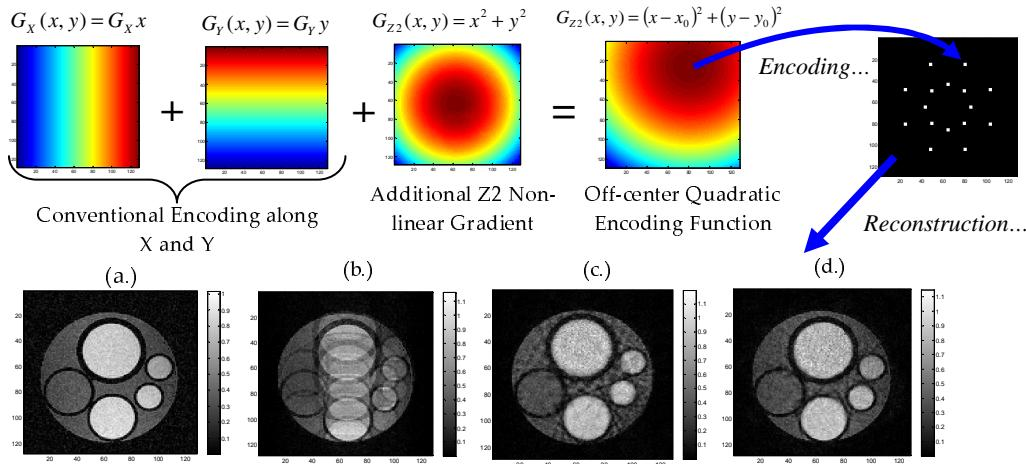
**ABOVE:** Using the Kaczmarz algorithm, 128x128 images are reconstructed from a reference image (a.) using three different 8-fold undersampled simulated datasets with 8 surface coils: Cartesian k-space data with 16 phase encode lines (a.), radial k-space data with 16 spokes (c.), and o-space with 16 CP’s (d.).
