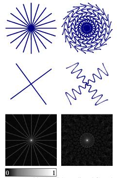
Fig 1: Traditional radial sampling (left) and oscillating radial sampling (right). Top row shows *k*-space sampling for ten radial arms. For clarity, second row displays only two of the ten radial arms shown in the first row. Third row shows PSF corresponding to the first row.
