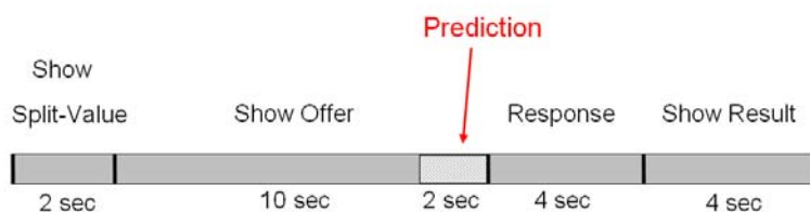
Fig. 1. The design of a single trial in the Ultimatum Game. The prediction of the decision is done 2 sec before the response phase, ensuring the result to be on hand before the actual response.
