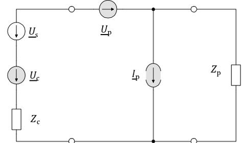
Fig. 1: Noisy single channel chain
