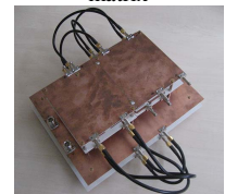
Fig. 2 Fabricated 8x8 Butler matrix for 300 MHz
