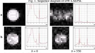
Fig. 2. DWSI of oscillating phantom using (a) DW-EPSI and (b) DW-LSEPSI. The left images show NAA maps.
