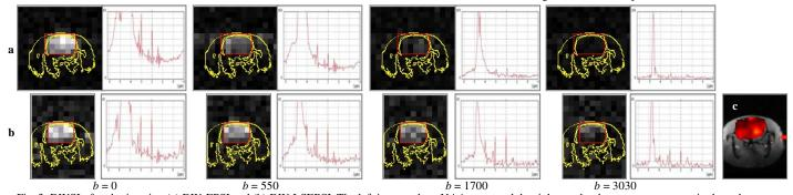
Fig. 3. DWSI of rat brain using (a) DW-EPSI and (b) DW-LSEPSI. The left images show NAA maps and the right graphs show average spectra in the red rectangles in the left images. Yellow lines in the left images show edges of a rat head. (c) ADC map of NAA using DW-LSEPSI. Color represents ADC value.
